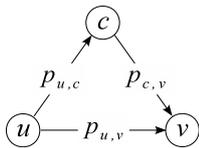
**Figure 1: One-hop transmission from node  $u$  to node  $v$  using node  $c$  for cooperative retransmission.**
