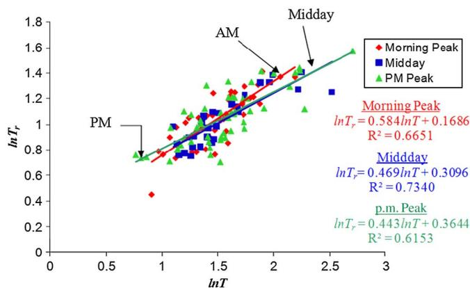
Fig. 5. Two-fluid model for different times of day for Orlando
