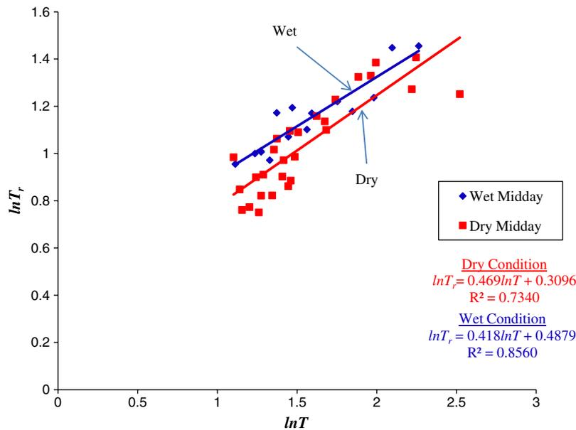
Fig. 4. Two-fluid model data for wet and dry pavement during the midday peak
