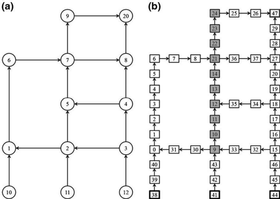
**Fig. 1** a Network used for numerical results b Equivalent cell network with higher capacity cells highlighted
