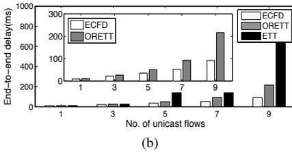
Fig. 4: Delay performance of unicast flows vs traffic load.
