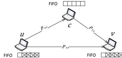
Fig. 1: A link from node  $u$  to node  $v$  using node  $c$  for cooperative retransmission.
