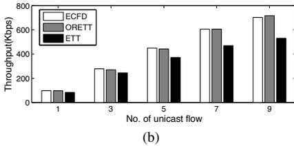
Fig. 3: Throughput of unicast flows vs traffic load.
