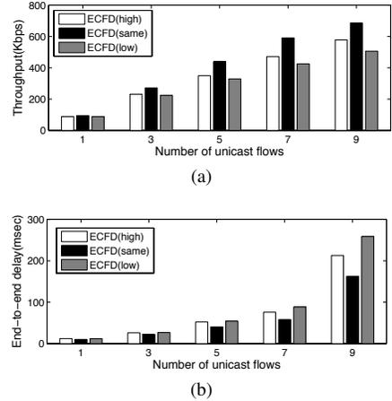
Fig. 2: Throughput and end-to end delay of unicast flows vs varying priority schemes.
