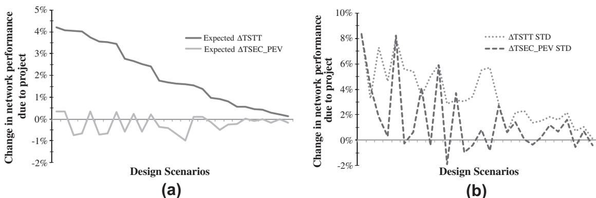
**Fig. 6.** Comparison of (a) expected system performance improvement and (b) variability of system performance for different design scenarios under stochastic demand for Sioux Falls.
