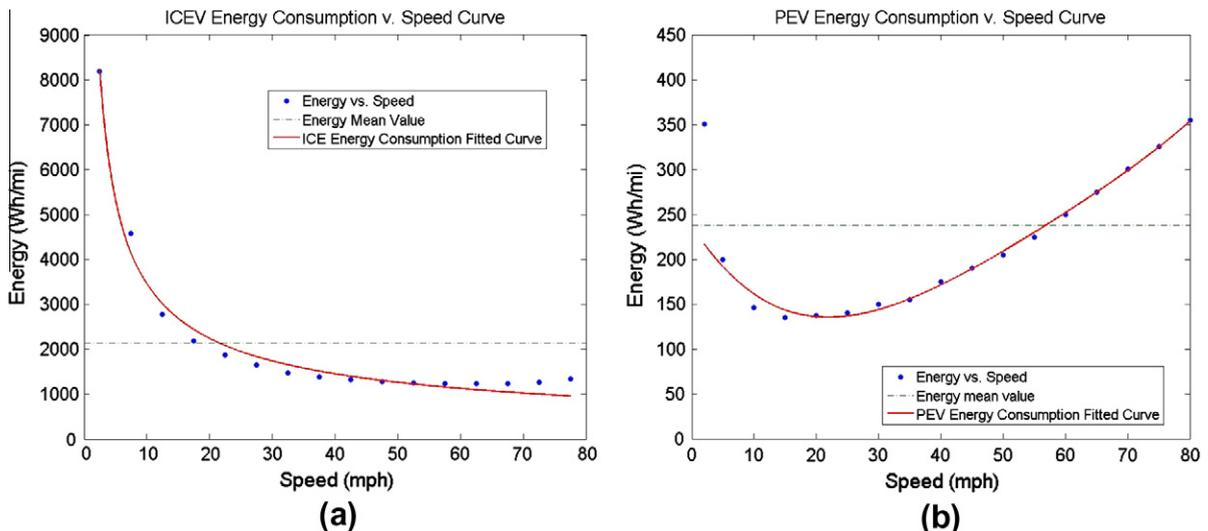
Fig. 2. Comparison of functional form of (a) ICEV energy consumption vs. (b) PEV energy consumption.
